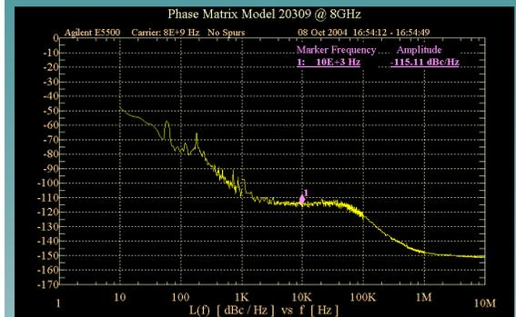
Phase Noise at 4 GHz and 8 GHz. Phase noise of better than -100dBc/Hz at a 10kHz offset make the 20309 the ideal L.O. for radar/EW testing.
